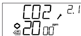
Example, Menu 2.1 CO 2 -control with input signal 0...10 V for CO 2 value 0...2000 ppm.
